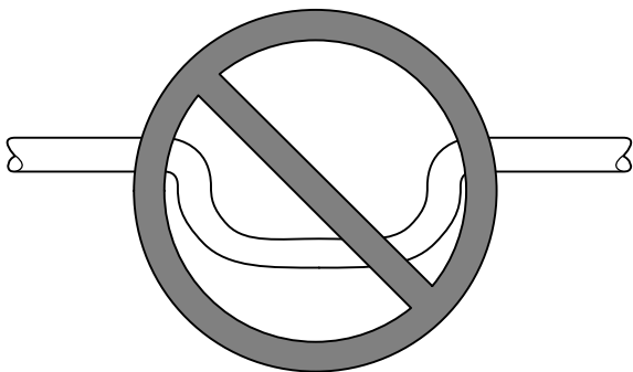
Figure 17 Insufficient Condensate Trap
